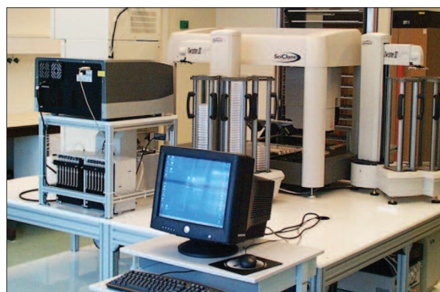
Figure 1. Robotic systems, shown at Dyadic's Netherlands subsidiary, are used for eukaryotic gene discovery by functional expression. (Top) Caliper LifeSciences' Allegro™ system is used for seeding microtiter plates with gene expression libraries, and for compression and replication of the libraries. After incubation of 96- or 384-well plates for growth and gene expression, the replicate (daughter) plates are assayed for proteins of interest using Caliper's Staccato™ system shown at bottom.
