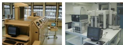
Fig 1: The Zymark Allegro library seeding, compression and replication station (left) and Staccato assay station (right) at DNL facility in Zeist.
